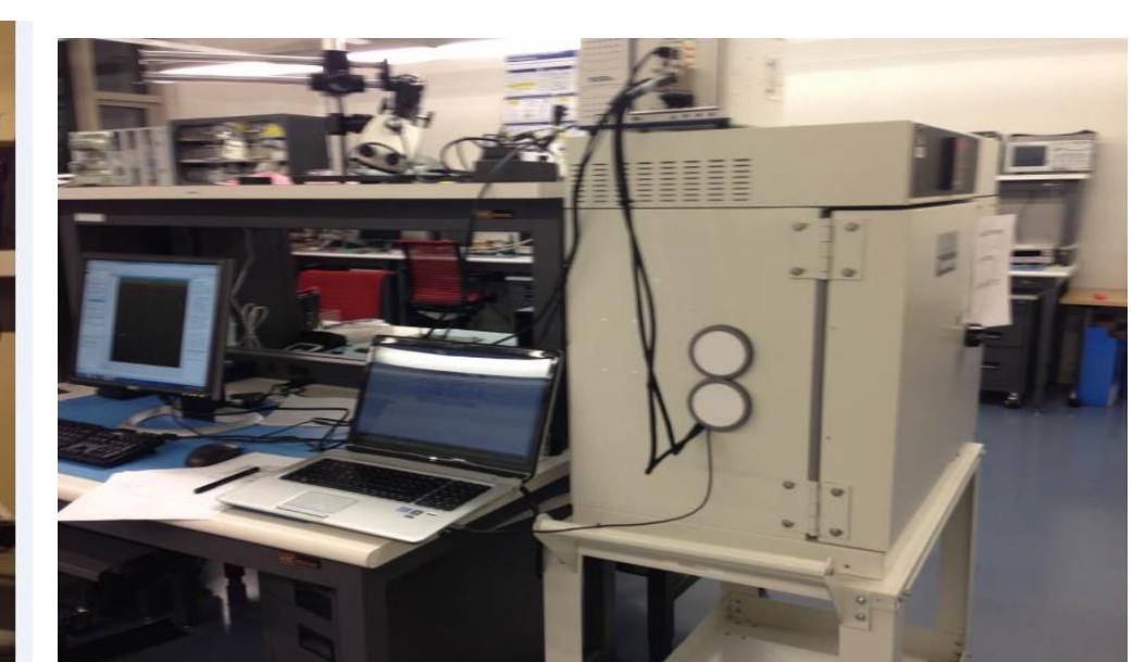
Temperature characteristic measurement In Thermal Chamber
